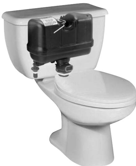
The solution was to retrofit the original pressure-assist toilets with the new 1.28 gpf *FLUSHMATE III* pressure-assist vessels, which converted them to High Efficiency Toilets (HET). The HET vessel provides a 20% reduction in consumption from the existing 1.6 gpf pressure vessel, while maintaining high performance. Upgrading to HET-classified toilets also can assist in attaining points for the U.S. Green Building Council's Leadership in Energy and Environmental Design (LEED) program.
